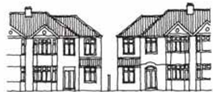
Side extensions subordinate to original dwellings and set in from boundary by 1m
