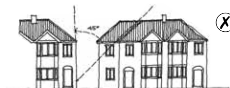
Overpowering extension causing loss of light to neighbour's protected side window
