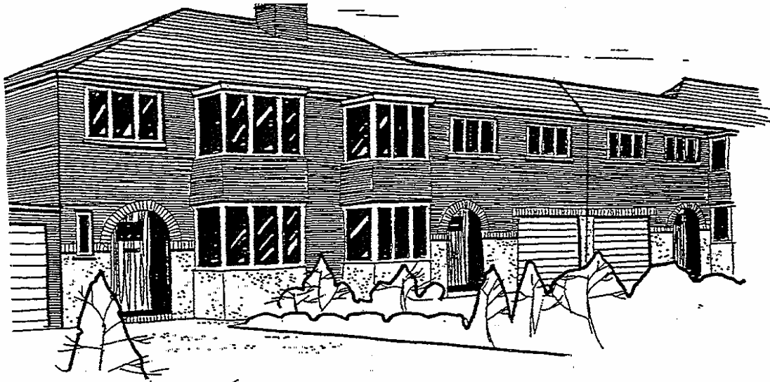
✘ Terracing effect where properties originally built as semi-detached
