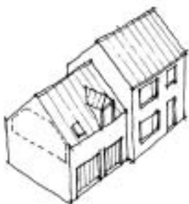
Extension subservient in form, emphasised by attic storey over garages. Smaller scale also reflected in separate openings for each car.
