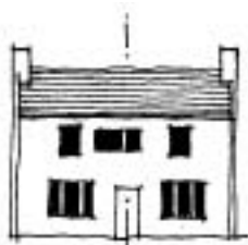
inappropriate window inserted without recognising symmetrical facade or vertical window proportions
