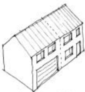
Extension dominates original house. This is emphasised by strong horizontals of double garage doors (often painted white).
