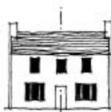
appropriate vertically proportioned window inserted on the centreline of the symmetrical facade
