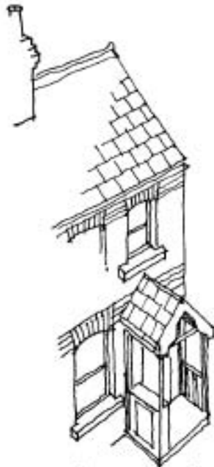
Open (or glazed) porch which reflects character of house, is spacious/open and incorporates meter box unobtrusively.
