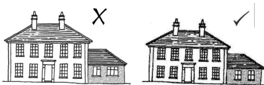
These windows are not sympathetic
