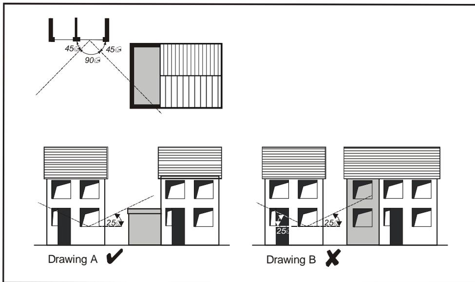
The extension shown above encroaches across the 45° line. However, if the extension is single storey only (drawing A) it does not cut across the 25° rising plane and is therefore acceptable, if a flat roof is visually also acceptable in this location. If the proposal is a two storey extension (drawing B) then it breaks the 25° rising plane and is unacceptable. The 25° angle is measured from cill level or the centre point of patio doors.
