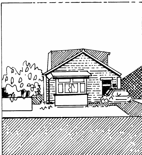
Fig. 9.5 Inappropriate Roof Extension
