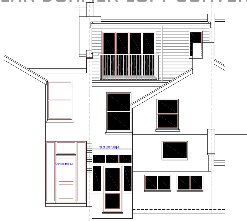
EXISTING REAR ELEVATION POST DEMOLITION 1:100 @ A3
